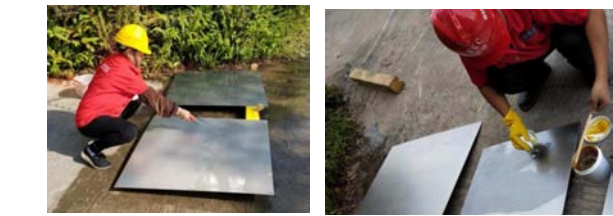
Figure 11. Pickling on outer surface of stainless steel.
