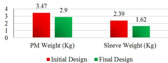
Figure 5. Comparison between the retention sleeve and the PM weights in the initial and the final design of HS-PMSG.
