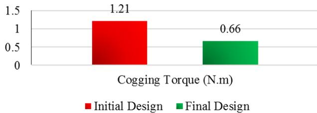
Figure 9. Comparison between cogging torque in the initial and the final design of HS-PMSG.
