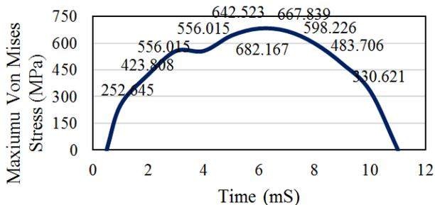
Figure 10. Maximum Von Mises stress in the rotor.
