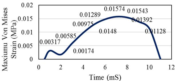
Figure 11. Maximum Von Mises strain in the rotor.
